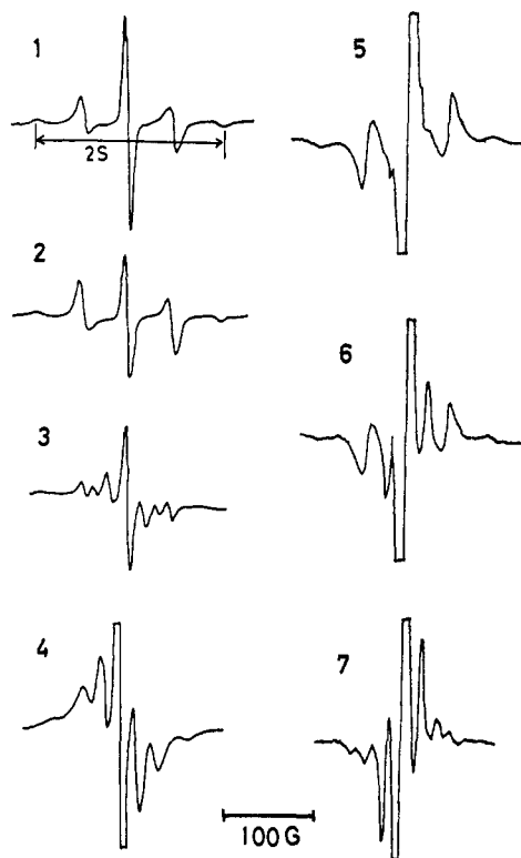
Figure 7. Rigid media epr spectra of alkali metal fluorenone ketyls. Sodium fluorenone: (1) \sim 10^{-2} M in MTHF, (2) \sim 10^{-3} M in MTHF, (3) \sim 5 \times 10^{-5} M in MTHF, (4) \sim 10^{-2} M in THF. Potassium fluorenone: (5) \sim 10^{-2} M in MTHF, (6) \sim 4 \times 10^{-4} M in MTHF, (7) \sim 8 \times 10^{-5} M in MTHF.
